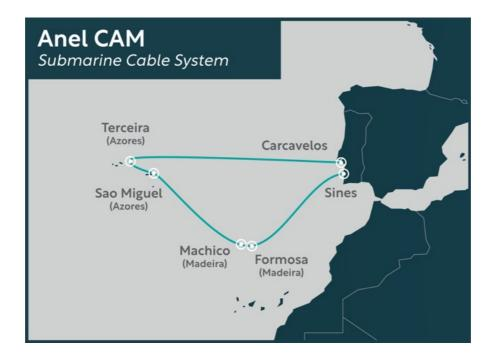
The new submarine cable system will be 3,812km long and comprise six pairs of optical fibers, offering a total capacity of at least 150 Tbps. This capacity represents a substantial increase on the current system, multiplying transmission capacity by 500 and ensuring ultra-high-speed, low-latency connectivity, essential for 5G mobile technologies and other services required by our digital economies.
