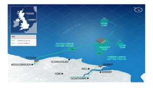
The DC/FO infrastructure will connect the onshore  $CO_2$  gathering network to subsea  $CO_2$  injection sites located approximately 145km from shore, enabling the delivery of power and communication to subsea control systems. The technology allows for future extensions, using the initially installed cable to connect additional manifolds as the volume of  $CO_2$  to be stored increases.
