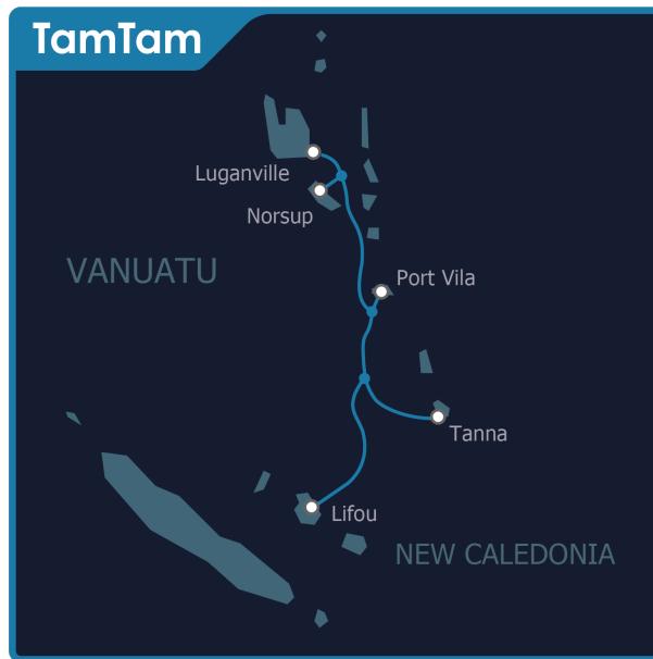
Map of the Tamtam Cable route connecting Vanuatu (Port Vila, Tanna, Norsup, Luganville) with New Caledonia (Lifou), including branching units (BU) along the route.
